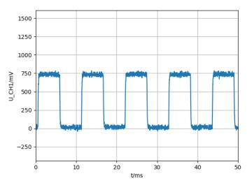
The sound is that of a typical rectangle signal, the absence of even harmonics makes it somewhat "hollow".
