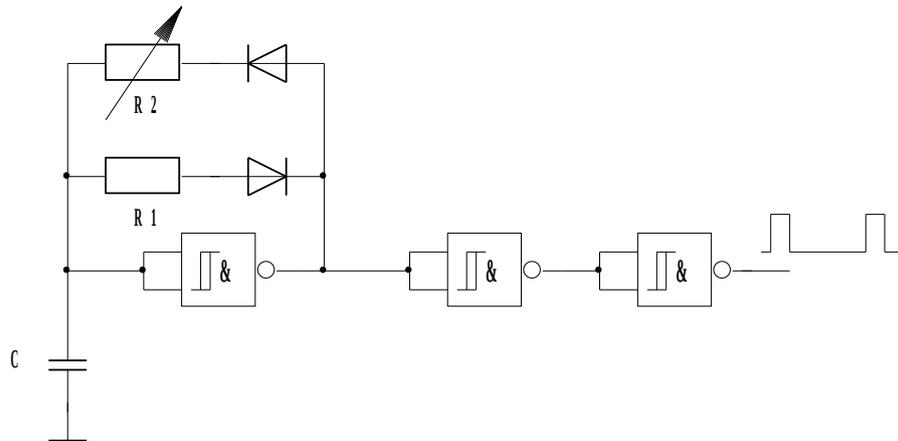
$R1 = 10\text{M}\Omega$ ,       $P1 = 250\text{k}\Omega$        $C = 10\text{nF}$
